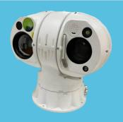
Birdlaser Gyro AI for use on movable platforms in aquaculture and marine environment will keep even stubborn seagulls away. Pan and tilt speed can be adjusted for optimal conditions and laser can be switched on and off by bird detection.
