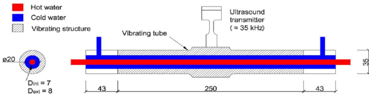
Figure 13: Heat exchanger design [15].
