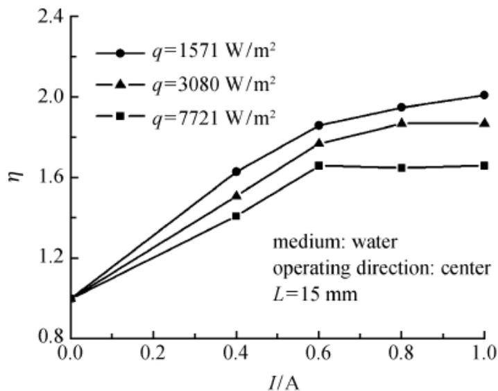
Figure 8: Enhancement ratio vs acoustic cavitation intensity [7].
