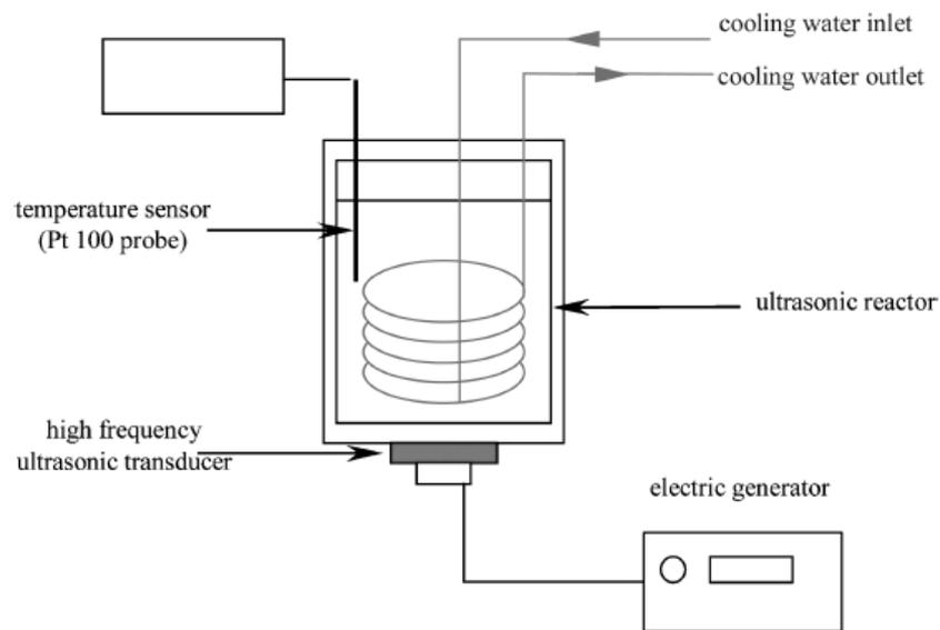
Figure 9: Experimentall setup [10].
