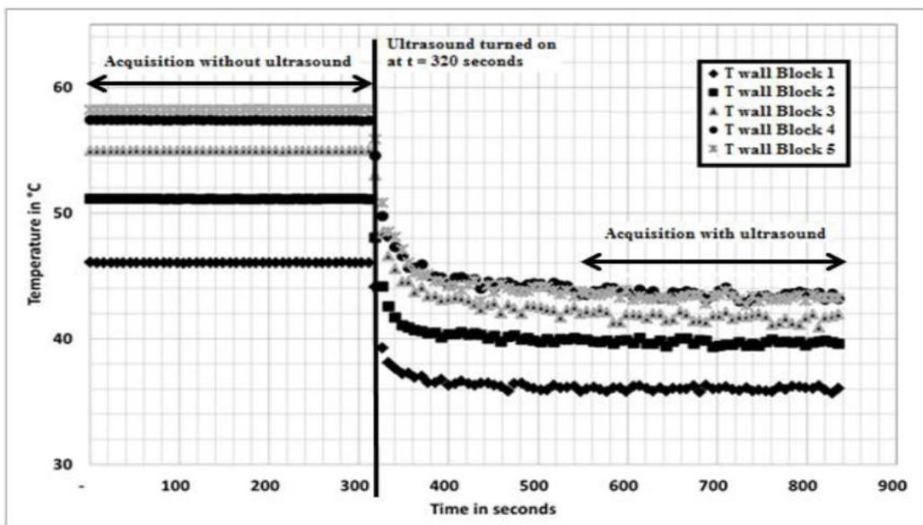
Figure 6: Wall temperature behaviour with respect to time [6].
