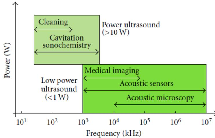
**Figure 2:** Usage of ultrasound [1].
