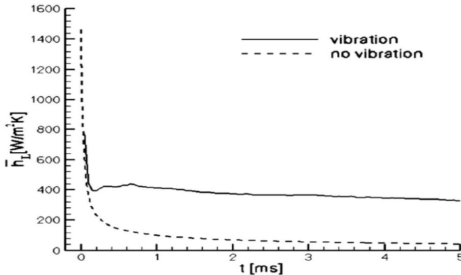
Figure 11: Average heat transfer coefficient with and without acoustic vibration [11].
