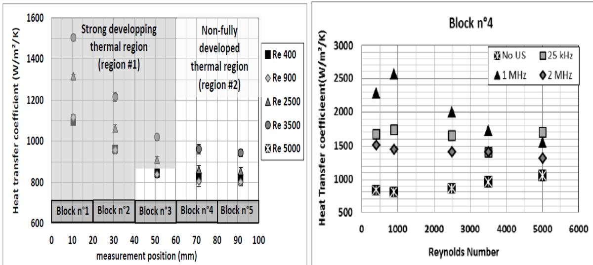
Figure 7a and 7b: Heat transfer coefficient with and without ultrasound at different location [6].
