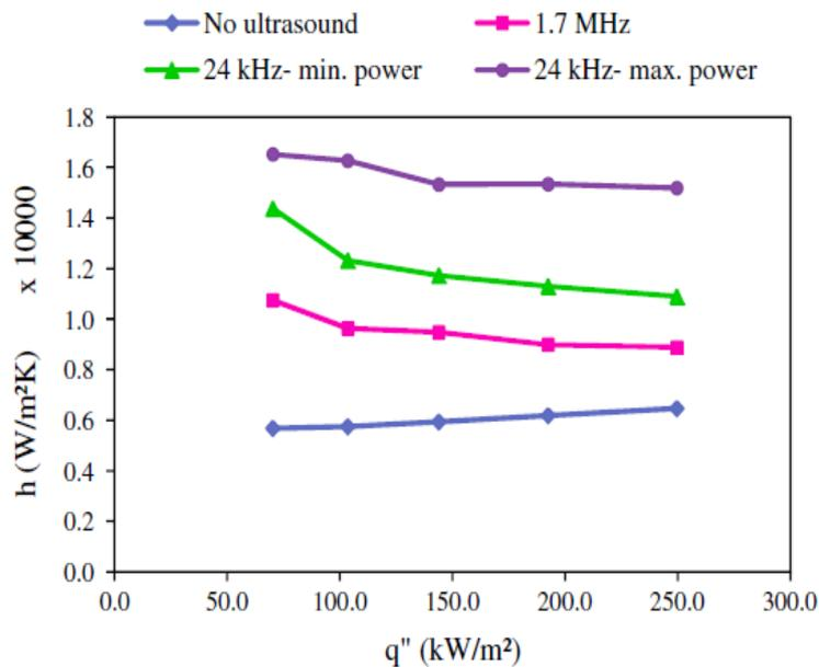
**Figure 4:** Heat transfer coefficient with changing ultrasound frequency and power [4].
